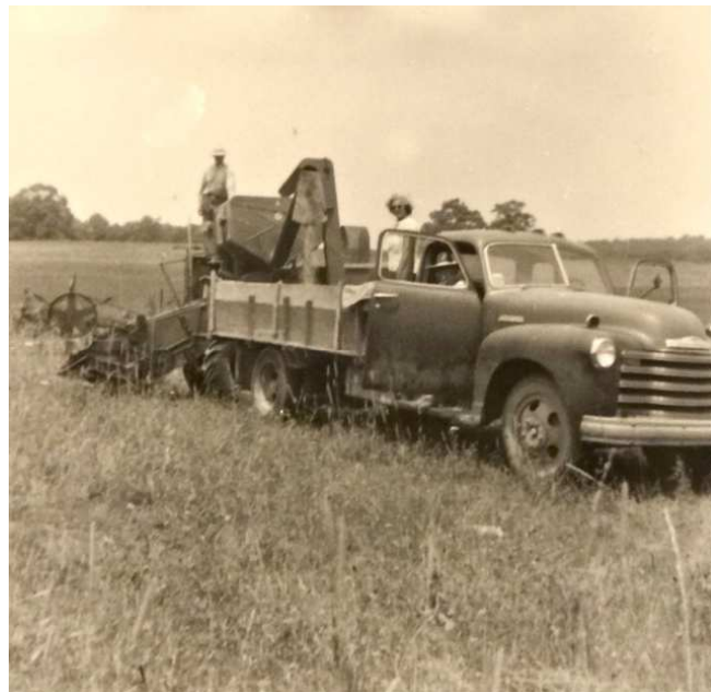
Self-propelled combine emptying grain from combine bin in to truck box in July.
