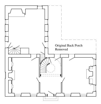
**Figure 21** First floor plan of the Thomas<sup>IV</sup> Barber house showing separation of front rooms and formal stair hall circulation from the back kitchen wing and service stairs.
