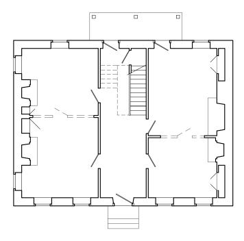
**Figure 15** First floor plan of the Samuel<sup>IV</sup> Barber house showing central hallway flanked by four rooms. The kitchen at right rear has a separate door to the back porch. (Long dash lines indicate original partitions which have been removed; short dashes show continuation of stairs and stairwell above).
