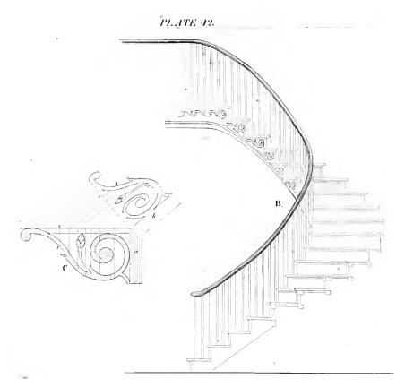
**Figure 31** Detail of circular stair from Biddle's *The Young Carpenter's Assistant*, an influential early 19<sup>th</sup> century builder's manual.<sup>53</sup> Biddle explained how to use geometry to lay out the carpentry of curved stairs.
