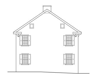
**Figure 16** Samuel<sup>IV</sup> Barber house in White Springs, drawing of south front and west gable elevations, showing original shutter and 12 over 12 window sash. The bracketed cornice **may be** a later alteration.
