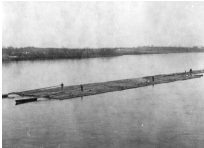
This undated view of a log “spar” raft on the Susquehanna River was taken from either the Market Street or Camelback Bridge. The raft is more than 100 feet long with at least eight distinct sections visible. A half-dozen men maneuver it downstream with huge sweeps. The logs likely originated from the robust logging industry in North Central Pennsylvania. Photo: Public Domain.
